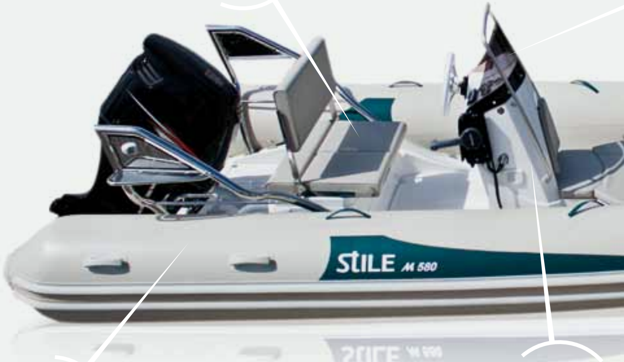
Consolle di guida completa di volante, timoneria, tientibene inox Console with steering wheel, steering system, stainless steel handrail
