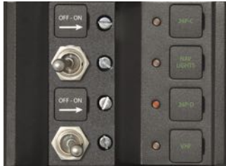
COTS Circuit Breaker (p. 80)
