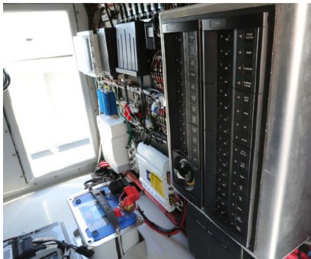
Metal Shark builds custom aluminum boats for government agencies. The Custom 360 Panel is housed inside the center console and distributes power to critical loads aboard the Relentless 28.
