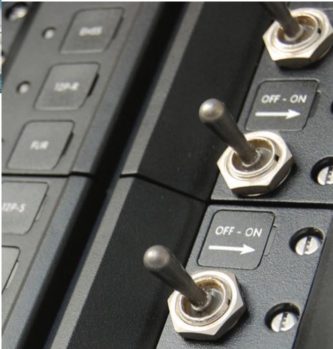
Metal Shark boats builds custom aluminum boats for government agencies. The Custom 360 Panel with Mil-Spec Toggle Circuit Breakers is housed inside the center console and distributes power to critical loads aboard the Relentless 28.
